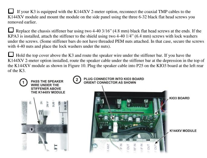
Figure 10. Connecting the Speaker Cable.
