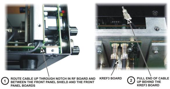
Figure 5. Routing the SMA Cable Behind the Front Panel.
