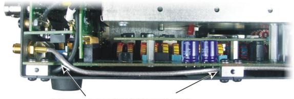
ROUTE CABLE THROUGH SLOT TO THE UNDERSIDE OF THE RF BOARD AND THEN BEHIND THE 2D FASTENER
