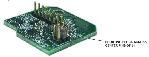
Figure 8. Shorting Block Installed on J1.
