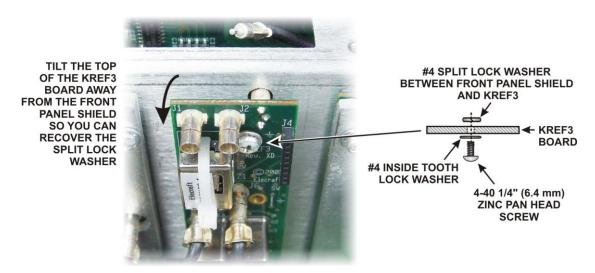
Figure 7. Removing the KREF3 Hardware.
