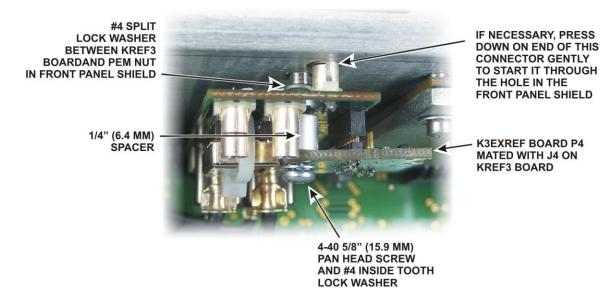
Figure 9. Mounting the K3EXREF Board on the KREF3 Board.
