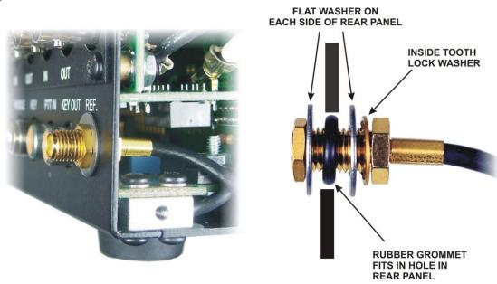
Figure 3. Mounting the SMA connector.
