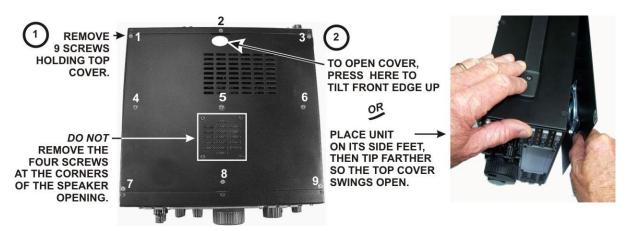
Figure 1. Removing K3 Top Cover.
